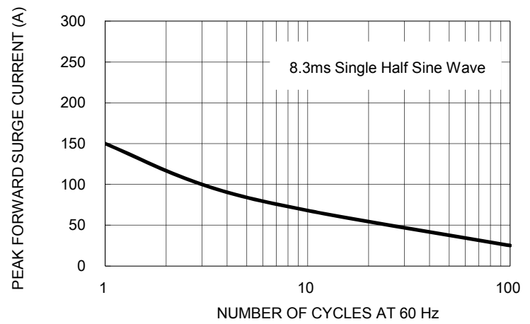
FIG. 2 MAXIMUM NON-REPETITIVE FORWARD SURGE CURRENT PER LEG
